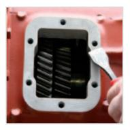
3. Rock the P.T.O driver gear in the transmission. This will show proper backlash of the transmission gears. This is only a guideline for feeling P.T.O. backlash (Later in Installation). NOTE: This should not replace checking backlash with a dial indicator measurement.
