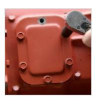
2. Keep aperture plate and bolts in safe place for future use. Clean pad around aperture hole with a gasket scraper. Note: Putting a rag in the aperture hole is recommended to prevent loose gasket material from entering the transmission.
